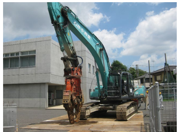
Photo 8 Current crushing attachment and heavy machine
