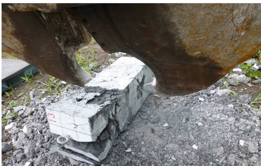
Fig. 13 A beam specimen of W/C=0.13 after repeated crushing loads showing the shortage of the crushing power.
