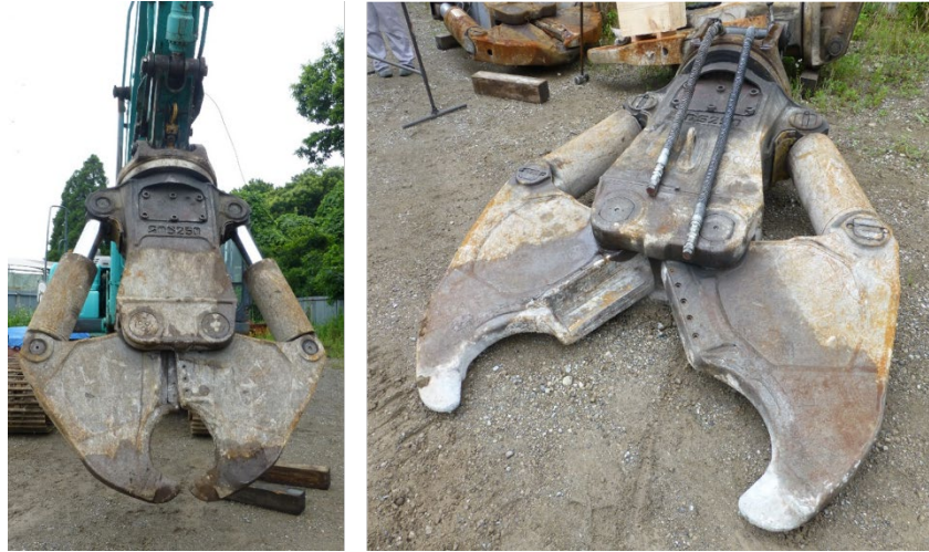
Fig. 10 Hydraulic shovel attachment.
