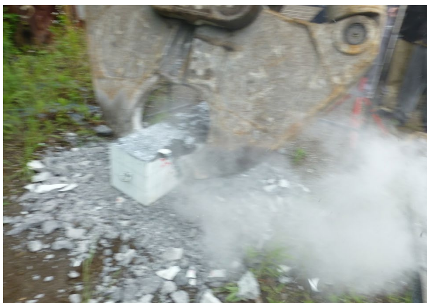
Fig. 12 Scatter of concrete pieces during crushing
